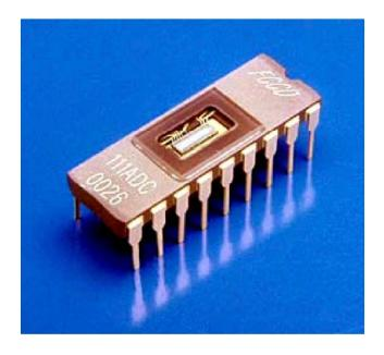
2-phase analog transport shift registers, an output charge detector/amplifier, and a compensation amplifier. The transport registers both feed the input of the charge detector resulting in sequential reading of the 256 sensing elements.
